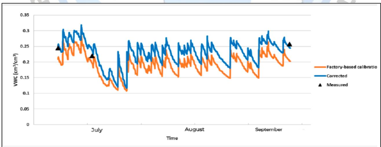
Figure 10: Comparison of factory-based calibration to corrected values for TDR in sand loamy
