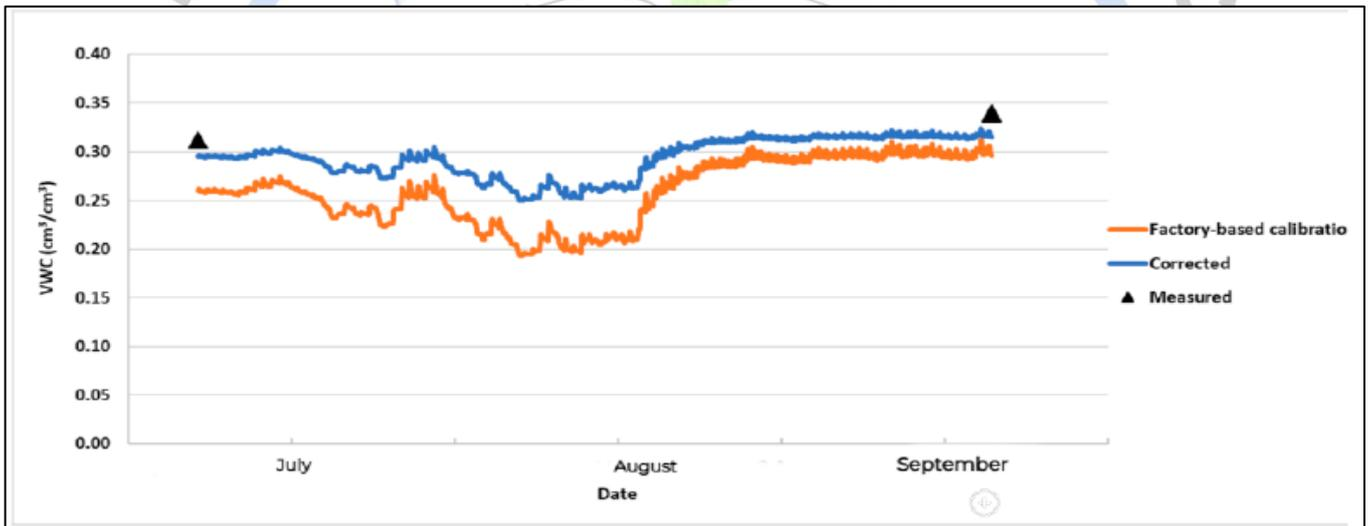
Figure 12: Comparison of factory-based calibration to corrected values for Resistive in sandy clay loam
