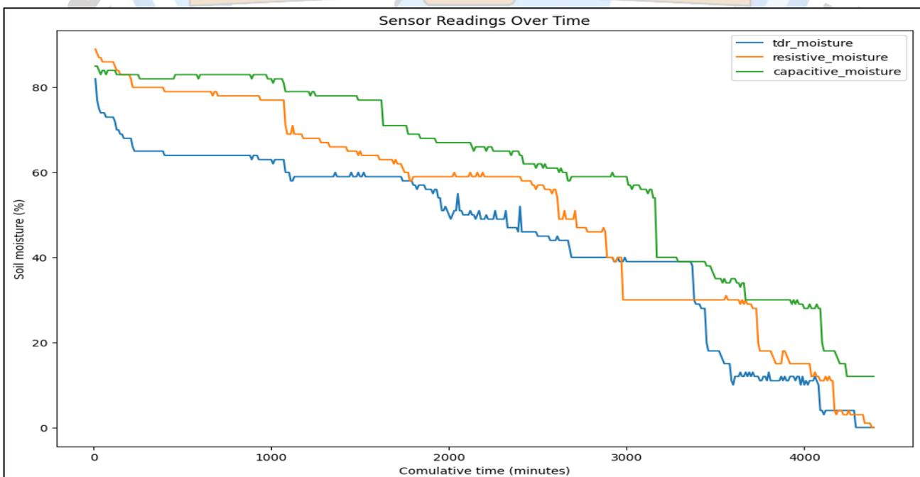
Figure 7: Sensor sensitivity comparison over time
