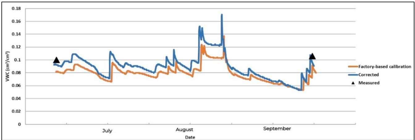
Figure 8: Comparison of factory-based calibration to corrected values for Capacitive in sand loamy
