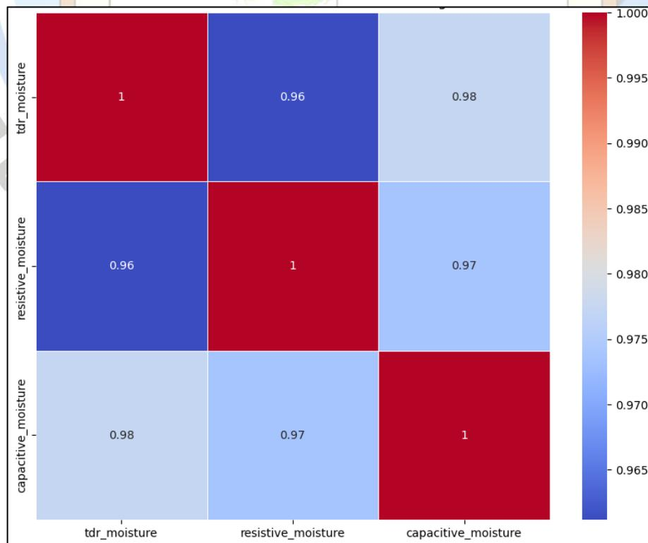
Figure 4: Correlation matrix of three sensors' moisture readings
