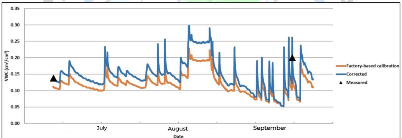
Figure 9: Comparison of factory-based calibration to corrected values for resistivity in sand loamy
