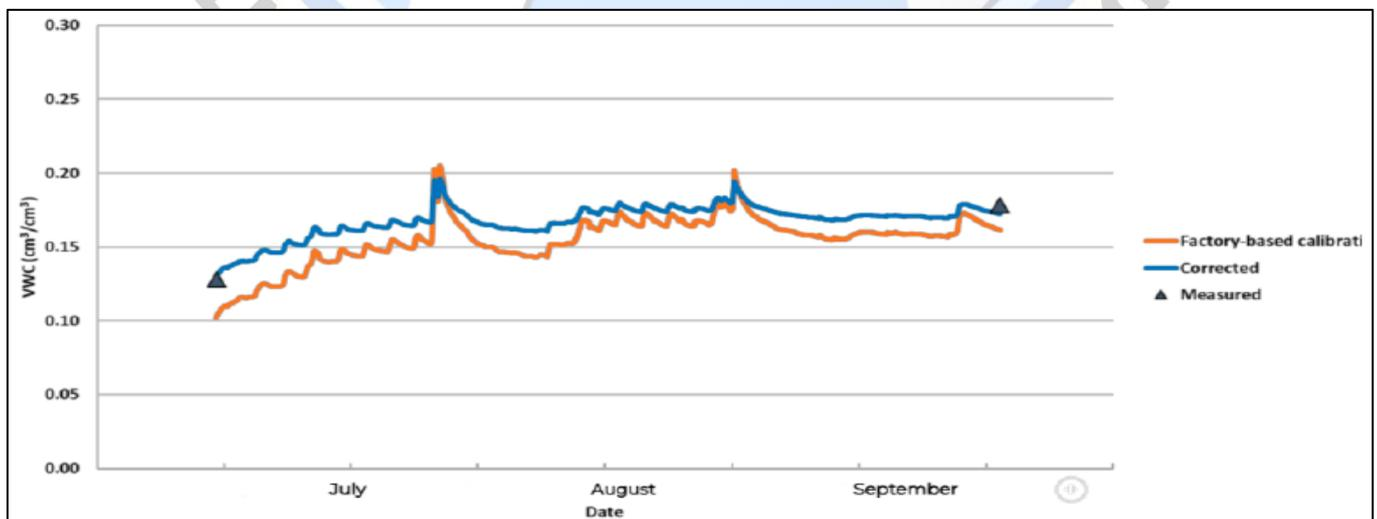
Figure 13: Comparison of factory-based calibration to corrected values for TDR in sandy clay loam
