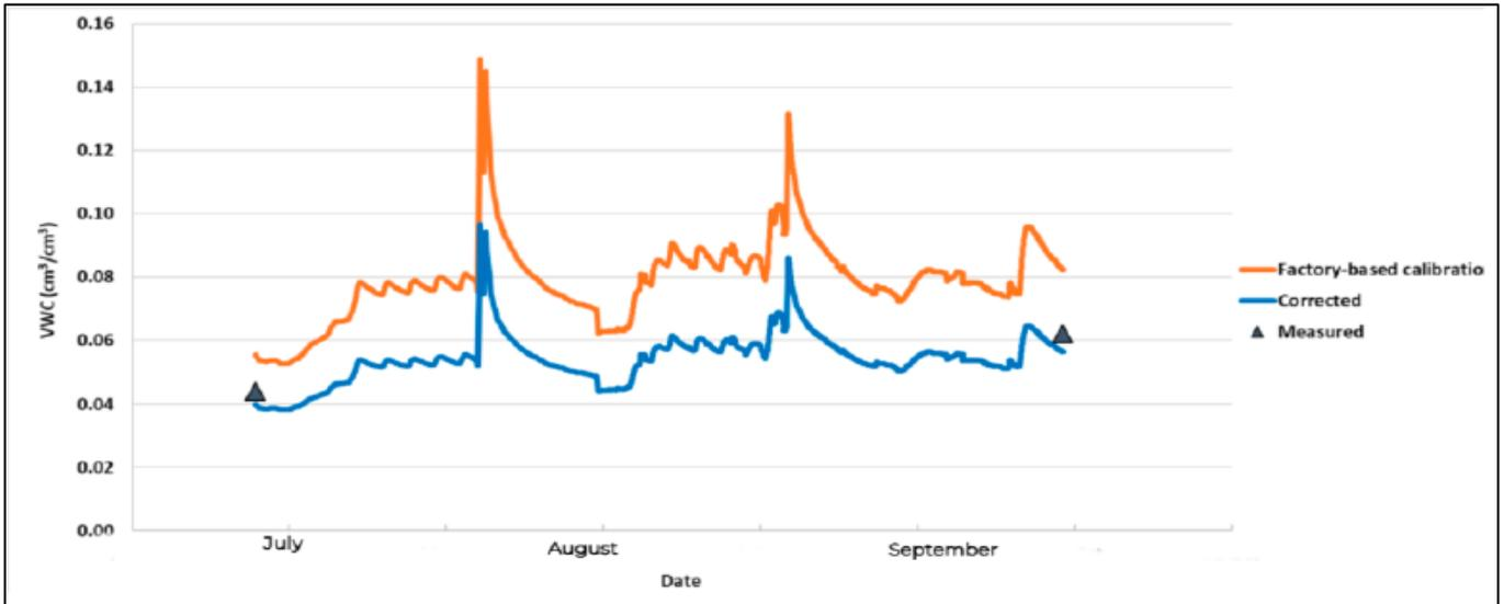
Figure 11: Comparison of factory-based calibration to corrected values for Capacitive in sandy clay loam
